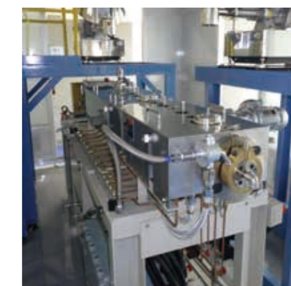
Twin-screw extruder with excellent performance in mixing high-viscosity substances and heat removal
